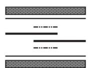
heating plate top silicone pad GST PU foil conveyor belt (conveying site up) conveyor belt (conveying site up) gauze + PU foil transparent silicone pad heating plate bottom
